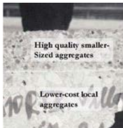
Figure 1: PCC over PCC, a type of composite pavement that lacks porosity (source: Tompkins & Darter, 2008)
